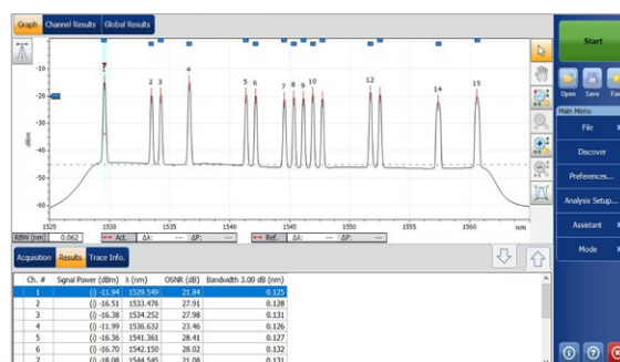
The FTBx-5235 displays channel power, channel wavelength and OSNR. Above: example of CWDM network OSA display. Below: example of DWDM network OSA display.
