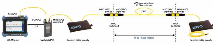
Figure 2: Typical test set-up for an unpinned-to-unpinned MPO trunk
