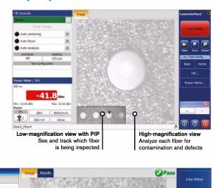
ConnectorMax2 also offers the smoothest MPO and MTP connector analysis process thanks to its unique PIP multifiber view, which is paired with the automated centering and focusing functions of the FIP-430/435. This leaves your hands free to control the X and Y scanning tool, enabling you to sequentially run the pass/fail analysis on each fiber of the connector in order to obtain a global status as per the standards.
