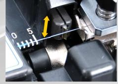
A new blade mechanism controls blade height automatically. It keeps good blade condition to obtain stable cleaving quality.
