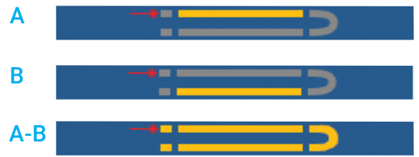
Using the loopback test method and iLOOP option on your iOLM enables you to test two fibers at once. View only the A link, B link, or the complete A-B link including the loop.
