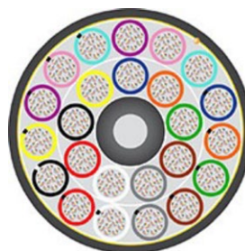
Example of a 3456 fibers cable.
