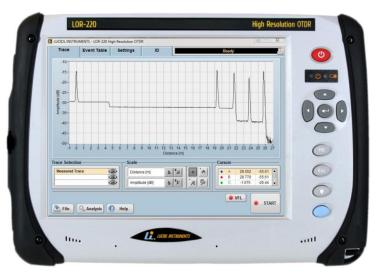
The LOR-220 from Luciol Instruments is a fully portable high resolution OTDR. It is similar in shape and feel to a standard OTDR but achieves unprecedented resolution.
