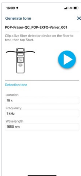
Figure 16: Tone activation for fiber identification.
