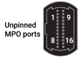
Figure 45: MPO-24 port configuration with 16 fibers
