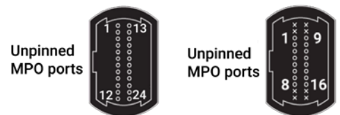
Figure 50: MPO-24 connectors with 24 fibers (left) or 16 fibers (right).
