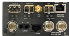
FTB-8130NG with next-generation SONET/SDH and OTN hardware including optical and electrical Ethernet add/drop interfaces.
