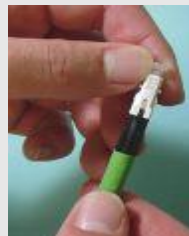
5) Push fit housing to complete
