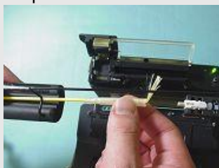
4) Assemble Heat Shrink
